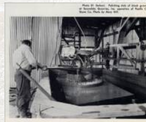
“Photo 81...Polishing slab of black granite at Escondido Quarries, Inc. operation of Pacific Cut Stone Co. Photo by Mary Hill.” (pp. 257)
